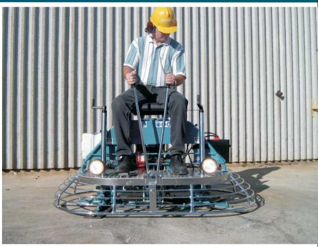
For the contractor who is considering the move to ride-on trowels our TS65 Ride-on Power Trowel is an easy step. The TS65 is an overlapping trowel based on our time tested B436 gearbox and spider plate assemblies. When you have found that walk behind trowels are no longer enough machine to get the job done make the step up to the TS65 Ride-on Power Trowel.
